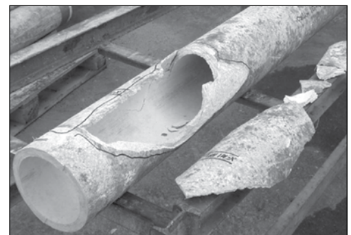
Corroded pipes like these will be replaced.
